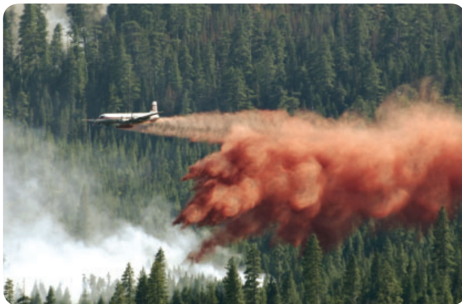
Figure 5 Fire retardants often contain chemicals to reduce cohesion and increase water’s ability to spread out and cover the burning material.
