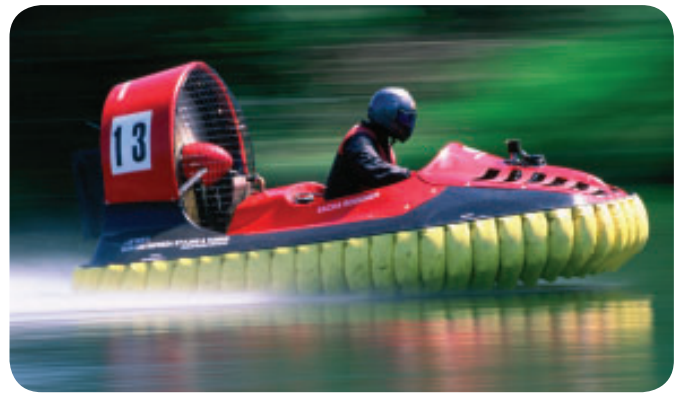
Figure 3 A hovercraft is a pneumatic system.
